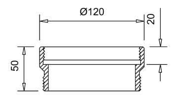
Frost Extension cast iron 20-40mm NPSM4
